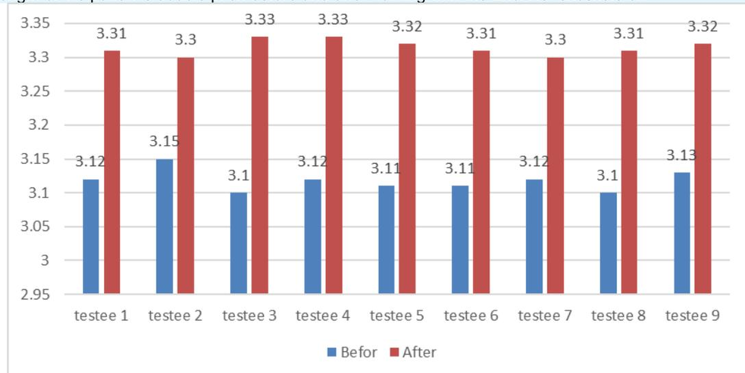
**Fig. 2.** Duration of the patients' walking cycle before and after training with the ExoAtlet exoskeleton
