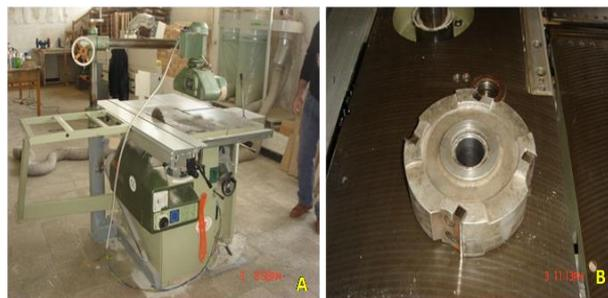
**Fig. 1.** A. General view of woodworking machine; B. Cutter head of Spindle Moulder and automatic feeding device
