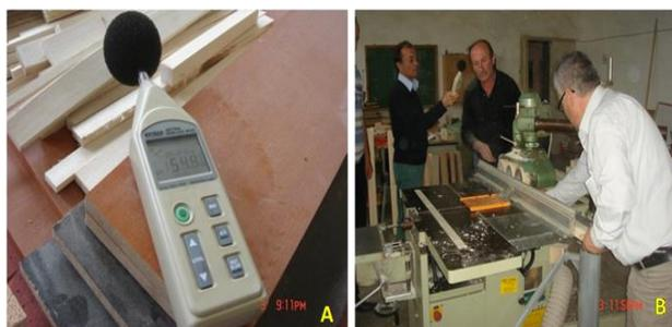
**Fig. 2.** A. Sound Level Meter EXTECH 407764; B) Measurements of Noise levels (dB)
