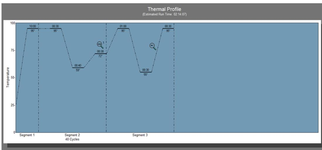
**Fig. 5.** Thermal profile used in *Eef2* Amplification. The image was taken directly from qPCR machine
